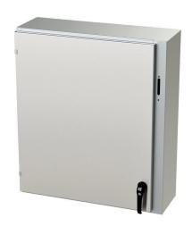
Saginaw Enviroline series disconnect enclosure, NEMA 3R/4/4X/12/13, right flange, 36 x 31 x 10in (HxWxD), wall mount, 316L stainless steel, #4 brush finish, single-door, 2-point padlocking handle, purchase subpanel separately.
