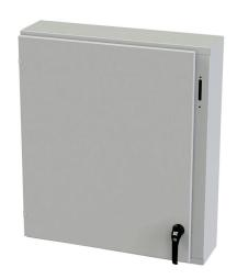
Saginaw Enviroline series disconnect enclosure, NEMA 3R/4/12/13, right flange, 36 x 31 x 8in (HxWxD), wall mount, carbon steel, RAL 7035 light gray, powder coat finish, single-door, 2-point padlocking handle, purchase subpanel separately.
