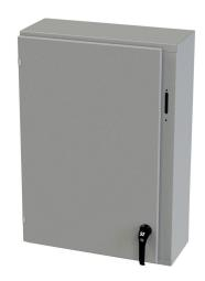
Saginaw Enviroline series disconnect enclosure, NEMA 3R/4/12/13, right flange, 36 x 25 x 10in (HxWxD), wall mount, carbon steel, ANSI 61 gray, powder coat finish, single-door, 2-point padlocking handle, purchase subpanel separately.
