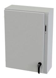
Saginaw Enviroline series disconnect enclosure, NEMA 3R/4/12/13, right flange, 36 x 25 x 10in (HxWxD), wall mount, carbon steel, RAL 7035 light gray, powder coat finish, single-door, 2-point padlocking handle, purchase subpanel separately.
