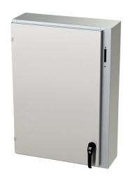
Saginaw Enviroline series disconnect enclosure, NEMA 3R/4/4X/12/13, right flange, 36 x 25 x 8in (HxWxD), wall mount, 304 stainless steel, #4 brush finish, single-door, 2-point padlocking handle, purchase subpanel separately.
