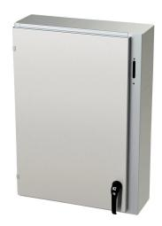
Saginaw Enviroline series disconnect enclosure, NEMA 3R/4/4X/12/13, right flange, 36 x 25 x 8in (HxWxD), wall mount, 316L stainless steel, #4 brush finish, single-door, 2-point padlocking handle, purchase subpanel separately.
