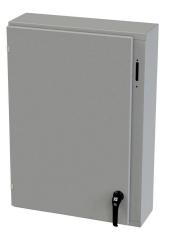
Saginaw Enviroline series disconnect enclosure, NEMA 3R/4/12/13, right flange, 36 x 25 x 8in (HxWxD), wall mount, carbon steel, ANSI 61 gray, powder coat finish, single-door, 2-point padlocking handle, purchase subpanel separately.
