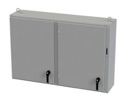
Saginaw disconnect enclosure, NEMA 3R/4/12/13, right flange,  $36 \times 54 \times 12$ in (HxWxD), freestanding/wall-mount, carbon steel, ANSI 61 gray, powder coat finish, 2-door, 3-point padlocking handle, purchase subpanel separately.
