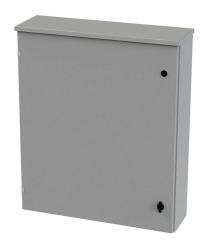
Saginaw enclosure, NEMA 3R, 36 x 30 x 8in (HxWxD), wall mount, carbon steel, ANSI 61 gray, powder coat finish, single-door, 1/4-turn padlocking wing handle.
