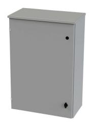
Saginaw enclosure, NEMA 3R, 36 x 24 x 12in (HxWxD), wall mount, carbon steel, ANSI 61 gray, powder coat finish, single-door, 1/4-turn padlocking wing handle.
