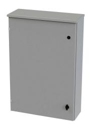
Saginaw enclosure, NEMA 3R, 36 x 24 x 8in (HxWxD), wall mount, carbon steel, ANSI 61 gray, powder coat finish, single-door, 1/4-turn padlocking wing handle.
