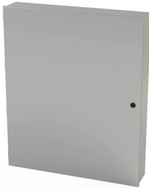
Saginaw enclosure, NEMA 1, 36 x 30 x 6in (HxWxD), wall mount, carbon steel, ANSI 61 gray, powder coat finish, single-door, 1/4-turn semi-flush latch.
