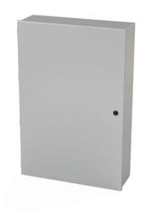
Saginaw enclosure, NEMA 1, 36 x 24 x 8in (HxWxD), wall mount, carbon steel, ANSI 61 gray, powder coat finish, single-door, 1/4-turn semi-flush latch.
