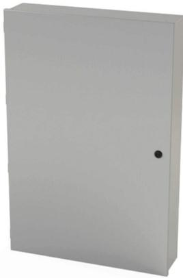
Saginaw enclosure, NEMA 1, 36 x 24 x 6in (HxWxD), wall mount, carbon steel, ANSI 61 gray, powder coat finish, single-door, 1/4-turn semi-flush latch.
