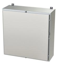
Saginaw enclosure, NEMA 3R/4/4X/12/13, 36 x 36 x 12in (HxWxD), wall mount, 316L stainless steel, #4 brush finish, single-door, stainless steel clamps, padlock hasp and staple.
