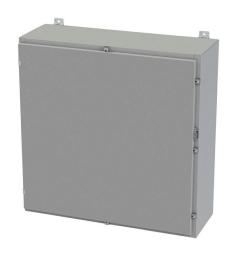
Saginaw enclosure, NEMA 3R/4/12/13, 36 x 36 x 12in (HxWxD), wall mount, carbon steel, ANSI 61 gray, powder coat finish, single-door, plated steel clamps, padlock hasp and staple.
