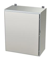
Saginaw enclosure, NEMA 3R/4/4X/12/13, 36 x 30 x 16in (HxWxD), wall mount, 304 stainless steel, #4 brush finish, single-door, stainless steel clamps, padlock hasp and staple.
