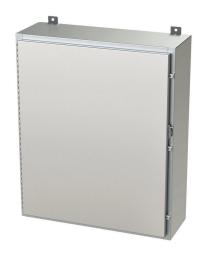
Saginaw enclosure, NEMA 3R/4/4X/12/13, 36 x 30 x 10in (HxWxD), wall mount, 304 stainless steel, #4 brush finish, single-door, stainless steel clamps, padlock hasp and staple.
