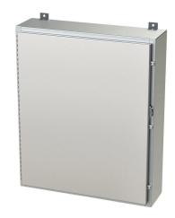
Saginaw enclosure, NEMA 3R/4/4X/12/13, 36 x 30 x 8in (HxWxD), wall mount, 304 stainless steel, #4 brush finish, single-door, stainless steel clamps, padlock hasp and staple.
