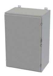
Saginaw enclosure, NEMA 3R/4/12/13, 36 x 24 x 16in (HxWxD), wall mount, carbon steel, ANSI 61 gray, powder coat finish, single-door, plated steel clamps, padlock hasp and staple.
