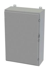
Saginaw enclosure, NEMA 3R/4/12/13, 36 x 24 x 10in (HxWxD), wall mount, carbon steel, ANSI 61 gray, powder coat finish, single-door, plated steel clamps, padlock hasp and staple.
