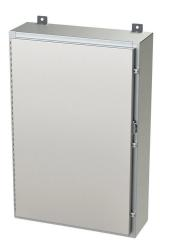
Saginaw enclosure, NEMA 3R/4/4X/12/13, 36 x 24 x 8in (HxWxD), wall mount, 304 stainless steel, #4 brush finish, single-door, stainless steel clamps, padlock hasp and staple.
