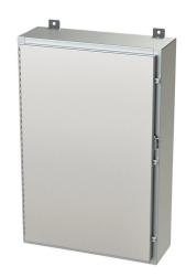
Saginaw enclosure, NEMA 3R/4/4X/12/13, 36 x 24 x 8in (HxWxD), wall mount, 304 stainless steel, #4 brush finish, single-door, stainless steel clamps, padlock hasp and staple.
