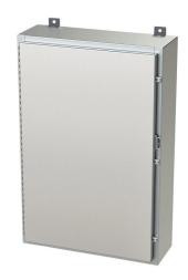
Saginaw enclosure, NEMA 3R/4/4X/12/13, 36 x 24 x 8in (HxWxD), wall mount, 316L stainless steel, #4 brush finish, single-door, stainless steel clamps, padlock hasp and staple.
