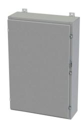
Saginaw enclosure, NEMA 3R/4/12/13, 36 x 24 x 8in (HxWxD), wall mount, carbon steel, ANSI 61 gray, powder coat finish, single-door, plated steel clamps, padlock hasp and staple.
