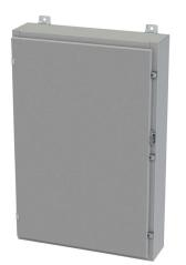
Saginaw enclosure, NEMA 3R/4/12/13, 36 x 24 x 6in (HxWxD), wall mount, carbon steel, ANSI 61 gray, powder coat finish, single-door, plated steel clamps, padlock hasp and staple.
