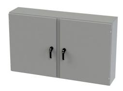
Saginaw Enviroline series enclosure, NEMA 3R/4/12/13, 36 x 60 x 12in (HxWxD), wall mount, carbon steel, ANSI 61 gray, powder coat finish, 2-door, 3-point keylocking/padlocking combo handle.
