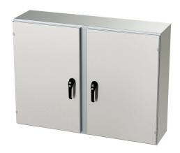
Saginaw Enviroline series enclosure, NEMA 3R/4/4X/12/13, 36 x 48 x 12in (HxWxD), wall mount, 304 stainless steel, #4 brush finish, 2-door, 3-point keylocking/padlocking combo handle.
