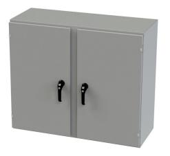
Saginaw Enviroline series enclosure, NEMA 3R/4/12/13, 36 x 42 x 16in (HxWxD), wall mount, carbon steel, ANSI 61 gray, powder coat finish, 2-door, 3-point keylocking/padlocking combo handle.
