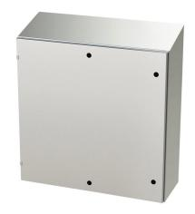
Saginaw Enviroline series enclosure, slope top, NEMA 3R/4/4X/12/13, 36 x 36 x 12in (HxWxD), wall mount, 304 stainless steel, #4 brush finish, single-door, 1/4-turn semi-flush latch.
