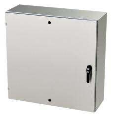
Saginaw Enviroline series enclosure, NEMA 3R/4/4X/12/13, 36 x 36 x 12in (HxWxD), wall mount, 304 stainless steel, #4 brush finish, single-door, 3-point keylocking/padlocking combo handle.
