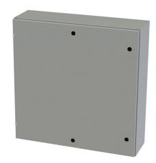
Saginaw Enviroline series enclosure, NEMA 3R/4/12/13, 36 x 36 x 10in (HxWxD), wall mount, carbon steel, ANSI 61 gray, powder coat finish, single-door, 1/4-turn semi-flush latch.
