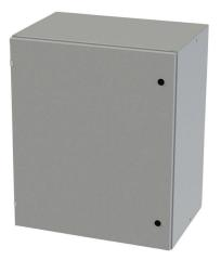
Saginaw Enviroline series enclosure, NEMA 3R/4/12/13, 36 x 30 x 20in (HxWxD), wall mount, carbon steel, ANSI 61 gray, powder coat finish, single-door, 1/4-turn semi-flush latch.
