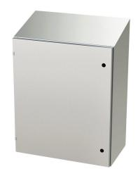
Saginaw Enviroline series enclosure, slope top, NEMA 3R/4/4X/12/13,  $36 \times 30 \times 16$  in (HxWxD), wall mount, 304 stainless steel, #4 brush finish, single-door, 1/4-turn semi-flush latch.
