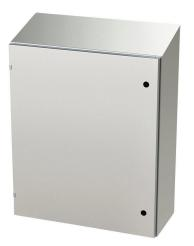
Saginaw Enviroline series enclosure, slope top, NEMA 3R/4/4X/12/13,  $36 \times 30 \times 12in$  (HxWxD), wall mount, 304 stainless steel, #4 brush finish, single-door, 1/4-turn semi-flush latch.
