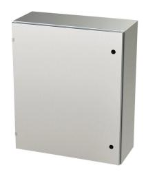
Saginaw Enviroline series enclosure, NEMA 3R/4/4X/12/13,  $36 \times 30 \times 12$ in (HxWxD), wall mount, 304 stainless steel, #4 brush finish, single-door, 1/4-turn semi-flush latch.
