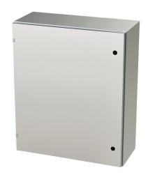
Saginaw Enviroline series enclosure, NEMA 3R/4/4X/12/13,  $36 \times 30 \times 12$ in (HxWxD), wall mount, 316L stainless steel, #4 brush finish, single-door, 1/4-turn semi-flush latch.
