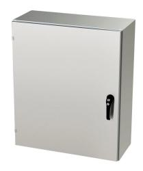
Saginaw Enviroline series enclosure, NEMA 3R/4/4X/12/13, 36 x 30 x 12in (HxWxD), wall mount, 316L stainless steel, #4 brush finish, single-door, 3-point keylocking/padlocking combo handle.
