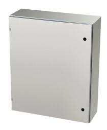
Saginaw Enviroline series enclosure, NEMA 3R/4/4X/12/13, 36 x 30 x 10in (HxWxD), wall mount, 304 stainless steel, #4 brush finish, single-door, 1/4-turn semi-flush latch.
