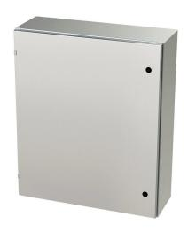
Saginaw Enviroline series enclosure, NEMA 3R/4/4X/12/13,  $36 \times 30 \times 10$ in (HxWxD), wall mount, 316L stainless steel, #4 brush finish, single-door, 1/4-turn semi-flush latch.
