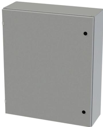
Saginaw Enviroline series enclosure, NEMA 3R/4/12/13, 36 x 30 x 10in (HxWxD), wall mount, carbon steel, ANSI 61 gray, powder coat finish, single-door, 1/4-turn semi-flush latch.
