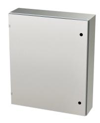
Saginaw Enviroline series enclosure, NEMA 3R/4/4X/12/13,  $36 \times 30 \times 8$  in (HxWxD), wall mount, 304 stainless steel, #4 brush finish, single-door, 1/4-turn semi-flush latch.
