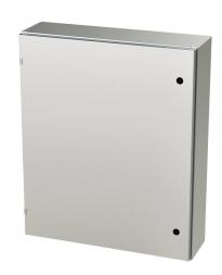
Saginaw Enviroline series enclosure, NEMA 3R/4/4X/12/13,  $36 \times 30 \times 8$  in (HxWxD), wall mount, 316L stainless steel, #4 brush finish, single-door, 1/4-turn semi-flush latch.
