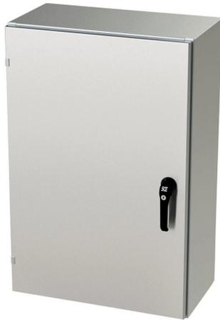
Saginaw Enviroline series enclosure, NEMA 3R/4/4X/12/13, 36 x 24 x 12in (HxWxD), wall mount, 316L stainless steel, #4 brush finish, single-door, 3-point keylocking/padlocking combo handle.
