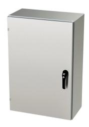
Saginaw Enviroline series enclosure, NEMA 3R/4/4X/12/13,  $36 \times 24 \times 12$  in (HxWxD), wall mount, 316L stainless steel, #4 brush finish, single-door, 3-point keylocking/padlocking combo handle.
