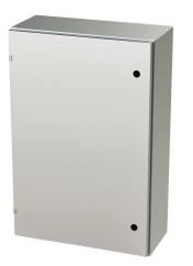
Saginaw Enviroline series enclosure, NEMA 3R/4/4X/12/13,  $36 \times 24 \times 10$  in (HxWxD), wall mount, 316L stainless steel, #4 brush finish, single-door, 1/4-turn semi-flush latch.
