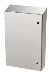
Saginaw Enviroline series enclosure, slope top, NEMA 3R/4/4X/12/13,  $36 \times 24 \times 8$  in (HxWxD), wall mount, 304 stainless steel, #4 brush finish, single-door, 1/4-turn semi-flush latch.
