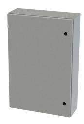
Saginaw Enviroline series enclosure, NEMA 3R/4/12/13,  $36 \times 24 \times 8$  in (HxWxD), wall mount, carbon steel, ANSI 61 gray, powder coat finish, single-door, 1/4-turn semi-flush latch.
