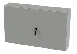
Saginaw enclosure, NEMA 3R/12/13, 36 x 60 x 12in (HxWxD), wall mount, carbon steel, ANSI 61 gray, powder coat finish, double-door, 3-point keylocking/padlocking combo handle.
