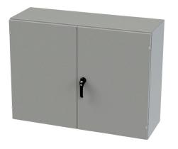
Saginaw enclosure, NEMA 3R/12/13, 36 x 48 x 16in (HxWxD), wall mount, carbon steel, ANSI 61 gray, powder coat finish, double-door, 3-point keylocking/padlocking combo handle.
