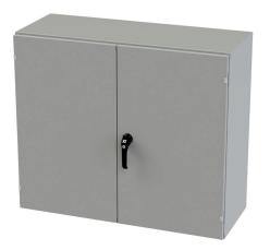
Saginaw enclosure, NEMA 3R/12/13, 36 x 42 x 16in (HxWxD), wall mount, carbon steel, ANSI 61 gray, powder coat finish, double-door, 3-point keylocking/padlocking combo handle.
