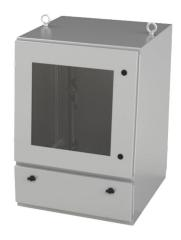
Saginaw workstation, NEMA 12/13, 34 x 24 x 24in (HxWxD), desktop or pedestal mount, dual access, carbon steel, RAL 7035 light gray, powder coat finish, single-door with keyboard drawer, 3-point keylocking flush swing handle, polycarbonate window.
